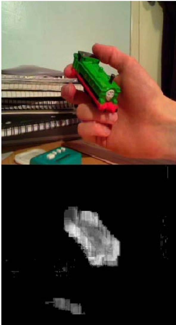
Fig. 5: The sliding window technique, using a Fast Unique Pixel Count filter. The upper image shows the camera image, and the lower image shows the output of the algorithm, searching for the signature of the toy train. The area of the object is clearly marked. Some noise is visible from other objects and details
