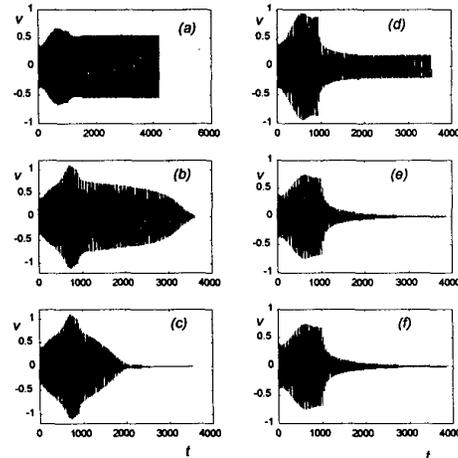
Figure 3. Numerical simulations of the time response, when  $f = 0.1$ ,  $\mu_1 = 0.01$ ,  $\lambda_2 = 0.01$ ,  $\alpha = -0.05$ .
