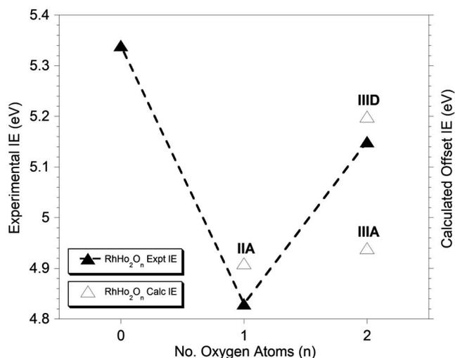
FIG. 5. Graph showing the experimental IE values for the  $\text{RhHo}_2\text{O}_n$  ( $n=0-2$ ) clusters as a function of constituent oxygen atoms. Also shown are the offset IE values calculated using DFT. Note that the “calculated offset” value for  $\text{RhHo}_2$  is arbitrarily set to the experimental value and this difference is used as the offset correction for the other calculated IE values. The isomer of each cluster that represents each IE value has also been labeled.
