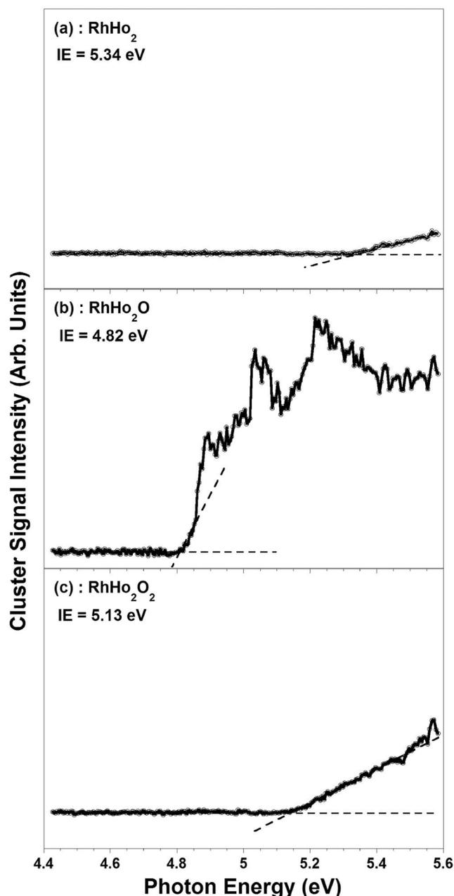
FIG. 3. PIE spectra of the RhHo<sub>2</sub>O<sub>n</sub> ( $n=0-2$ ) clusters. The determined IEs are also displayed (uncertainty in IEs =  $\pm 0.05$  eV).
