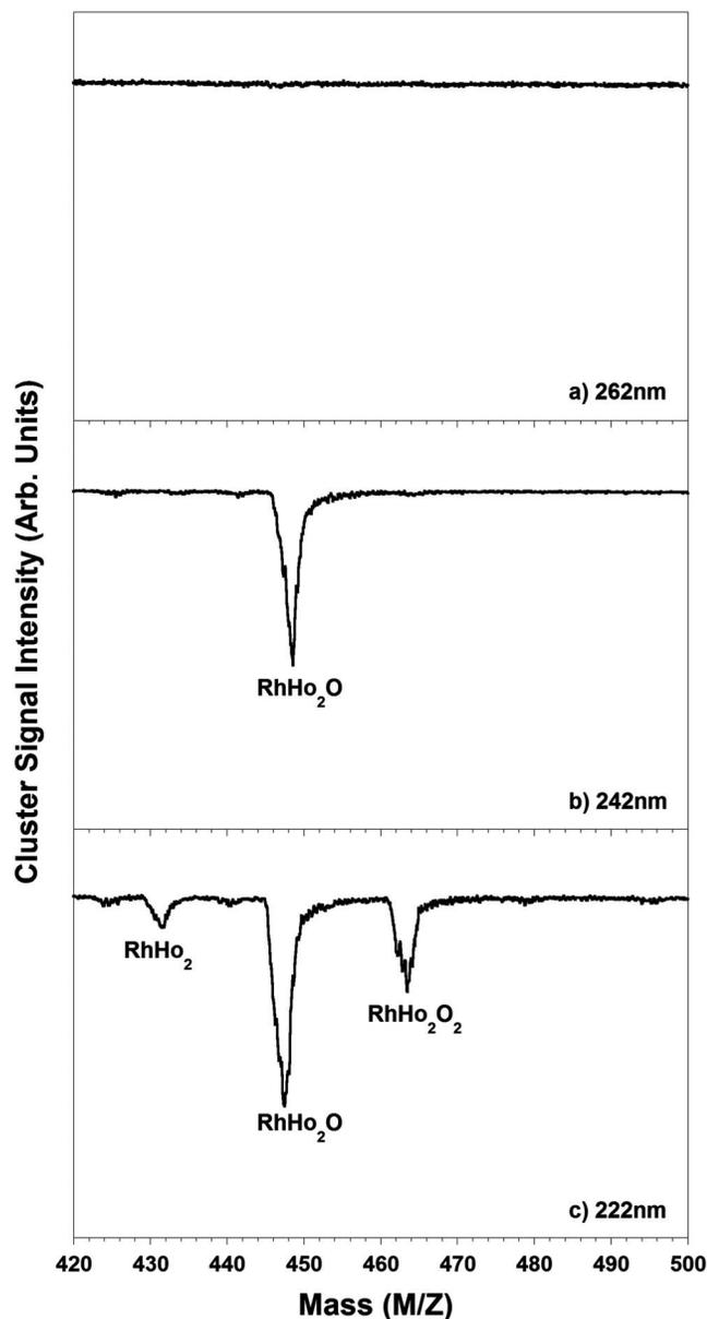
FIG. 2. Mass spectra of the RhHo<sub>2</sub>O<sub>n</sub> ( $n=0-2$ ) clusters recorded at three different ionization wavelengths: (a) 262, (b) 242, and (c) 222 nm.
