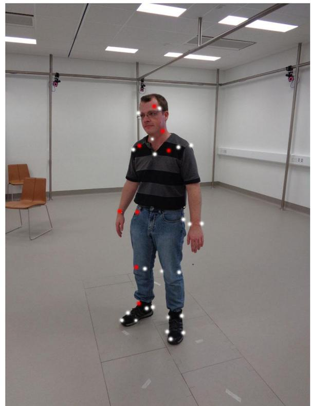
**Figure 3. Body with markers suitable for Maya pivot rigging (white markers are directly visible, red markers are included to indicate the corresponding marker that is masked or out of view). Note 3 of 10 Vicon Bonita cameras are visible in the background.**
