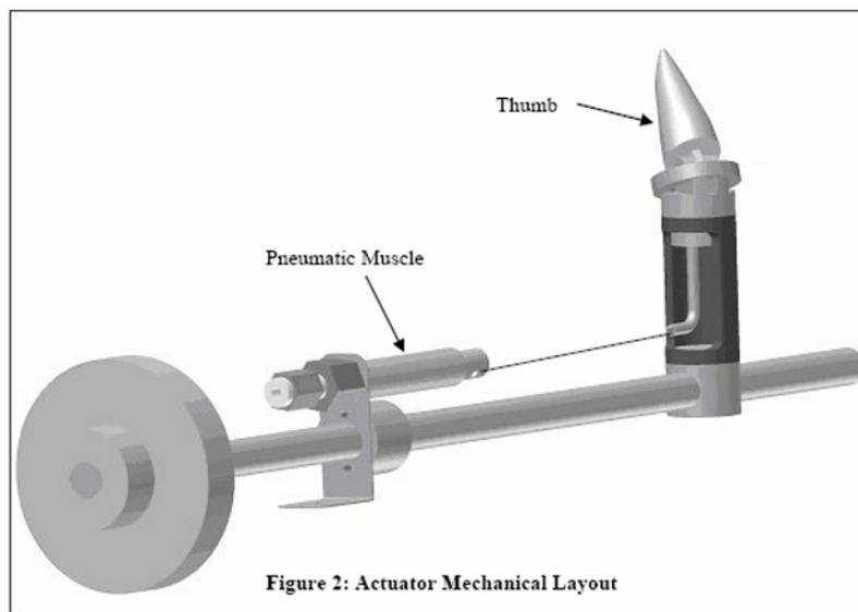
Figure 2: Actuator Mechanical Layout
